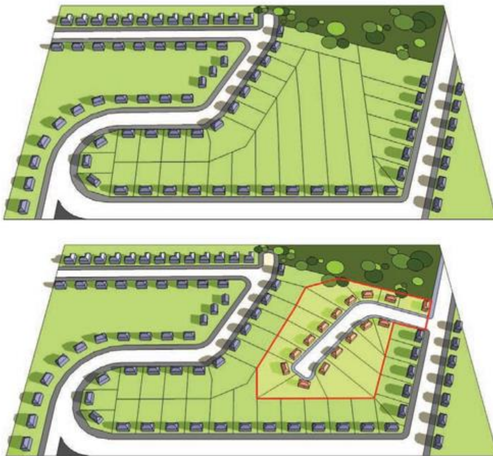
Figure 25 - Assembling a number of backland sites and developing them comprehensively can result in a more satisfactory form of development than would be achieved by individual competing backland / tandem schemes on neighbouring plots
