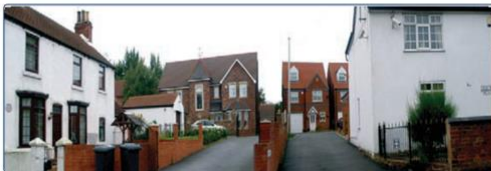
Figure 26 - Two poor quality, piecemeal backland developments have created multiple access points on this street frontage, increasing the prominence of the properties to the rear. The access road to the development on the right is located too close to the host property. In both developments, the new backland properties are significantly taller than the host properties and have little relevance to the traditional
