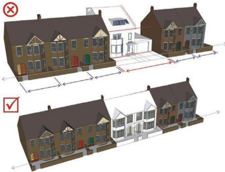
Figure 28 - Top: Insensitive contemporary infill includes: Plot width not respected; space created to the side of the property; House set back from existing building line; Depth of the property results in inappropriate roof pitch; Dormer window uncharacteristic of street; Open plan front garden not appropriate. Bottom: Sensitive contemporary infill: Plot width, building height, depth and roof pitch respected; No gaps between properties, building line maintained; Contemporary building elements mirror existing character; Full height bays and gables reflect existing; Fenestration pattern and rhythm compliment frontage; Front gardens and boundary treatment reinforce street.
